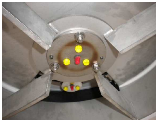
new stainless steel housing bearing arrangement
